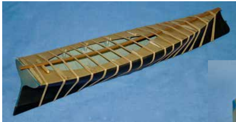
Above, elastic bands clamping the "flat" deck. Right, the planked, crowned deck with trial paper coaming.
