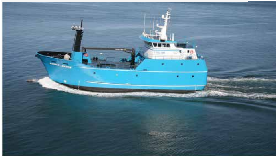
Steel hull Freezer Longliner "Bering Leader" after launching at Patti Industries' yard in Pensacola
