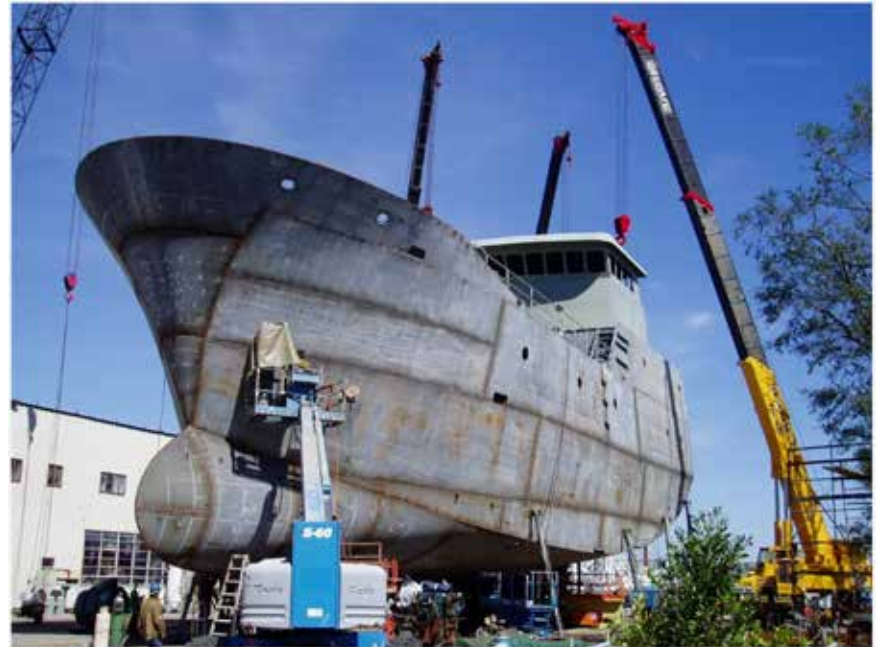
Construction of steel boat "Bering Leader" by Patti Industries Pensacola. Length: 124 feet, Beam: 40 feet, Draft: 16.6 feet
