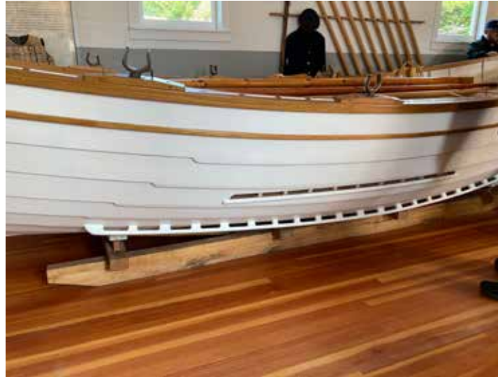
• Same boat showing drainage slots from inner deck.
