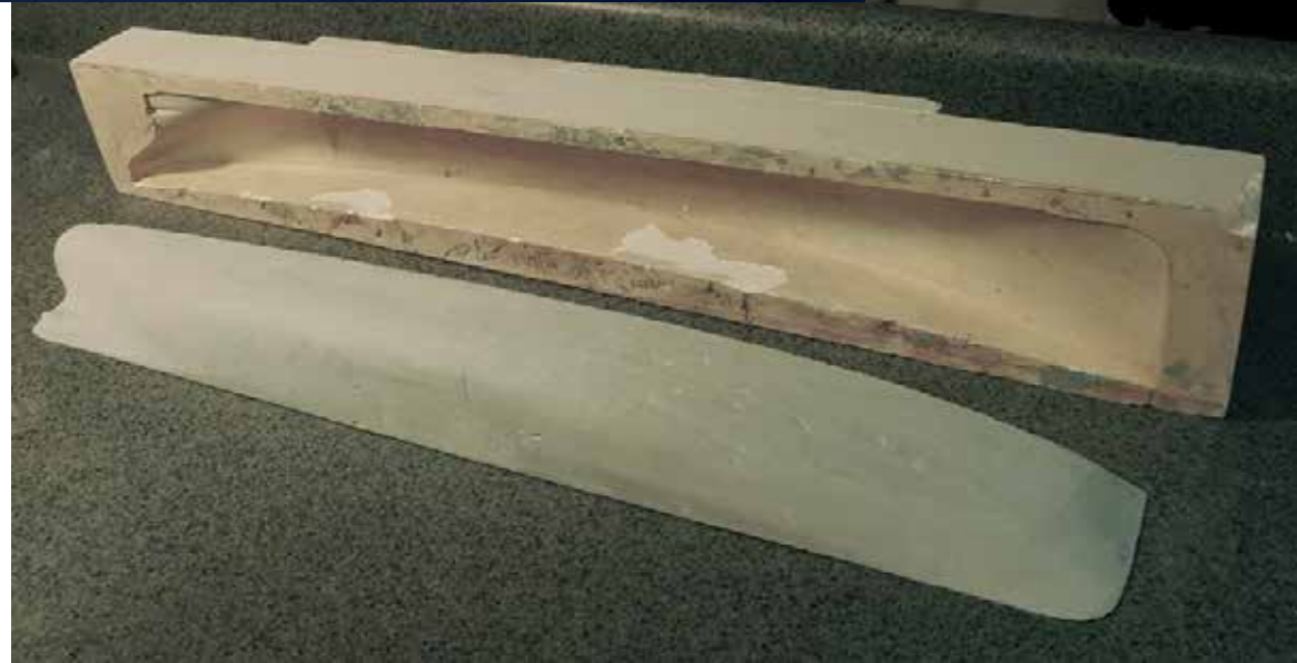
Above, my redraw of original shipyard hull plan, the 2017 foam pattern and the Plaster-of-Paris mold. At right, the 2024 Bondo casting, in the rough.
