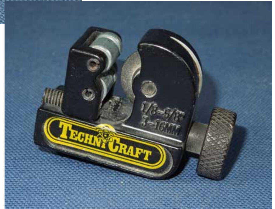
Sec/Ed's Tubing cutter. Would not work for very short lengths, due to the configuration of the rollers opposing the cutting wheel.
